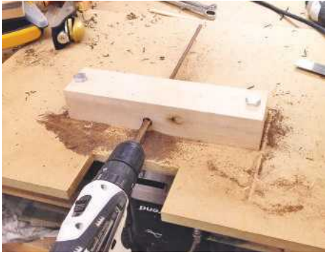
Custom-made dowels courtesy of a handheld drill and an ingenious jig that...
